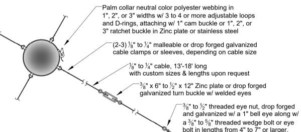
bolt in lengths from 4" to 7" or larger, depending on concrete wall thickness and load requirements w/ epoxy filling, if needed
