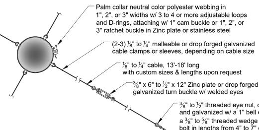
$^{-3}$ %" to  $^{1}$ 2" threaded eye nut, drop forged and galvanized w/ a 1" bell eye along w/ a  $^{3}$ 6" to  $^{5}$ 6" threaded wedge bolt or eye bolt in lengths from 4" to 7" or larger, depending on concrete wall thickness and load requirements w/ epoxy filling, if needed
