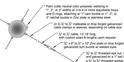
3/8" to 1/2" threaded eye nut, drop forged and galvanized w/ a 1" bell eye along w/ a 3/8" to 5/8" threaded wedge bolt or eye bolt in lengths from 4" to 7" or larger, depending on concrete wall thickness and load requirements w/ epoxy filling, if needed
