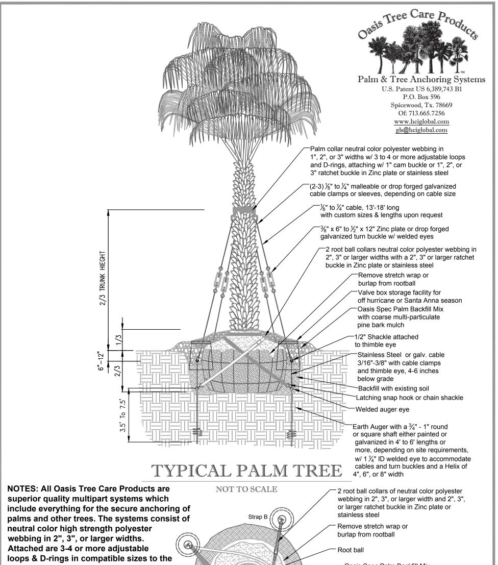
webbing with a 1" cam buckle or a 1", 2", or 3" Ratchet buckle. Cabling is 7x19 galvanized aircraft cable from  $\frac{1}{8}$ " to  $\frac{1}{4}$ " or
