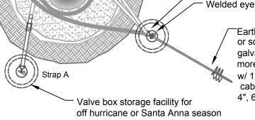
Earth Auger with a <sup>3</sup>/<sub>4</sub>" - 1" round or square shaft either painted or galvanized in 4' to 6' lengths or more, depending on site requirements, w/ 1 <sup>1</sup>/<sub>4</sub>" ID welded eye to accommodate cables and turn buckles and a Helix of 4", 6", or 8" width
