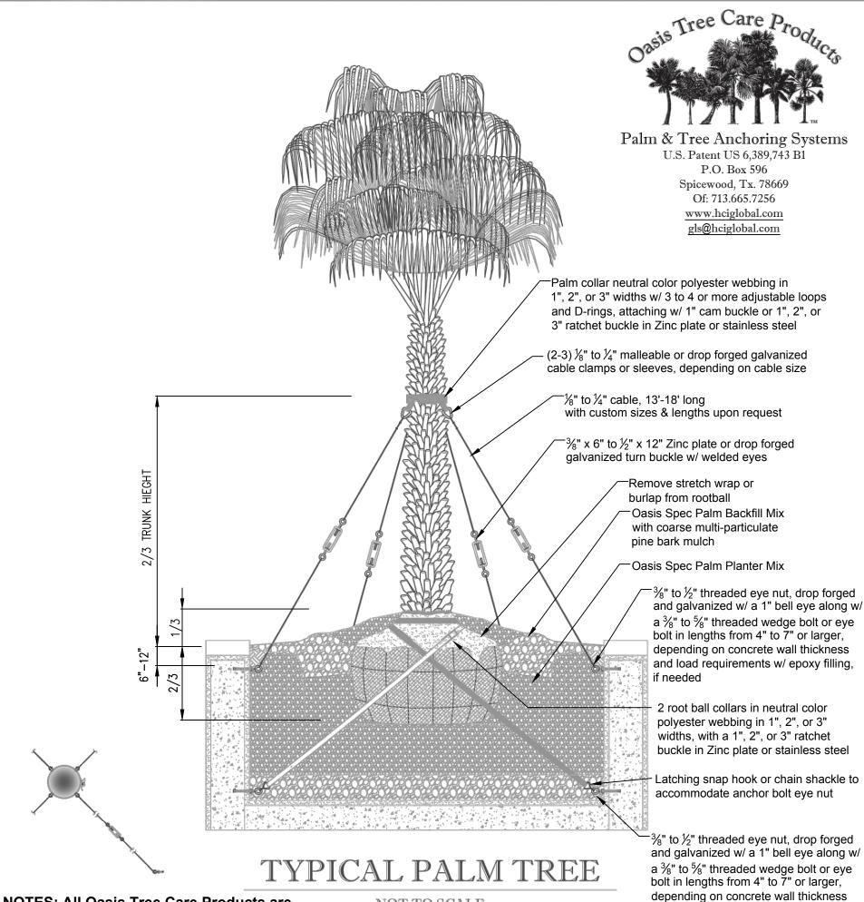
**NOTES: All Oasis Tree Care Products are** superior quality multipart systems which include everything for the secure anchoring of palms and other trees. The systems consist of neutral color high strength polyester webbing in 1", 2", and 3" widths. Attached are 3-4 or more adjustable loops & D-rings in compatible sizes to the webbing with a 1" cam buckle or a 1", 2",
